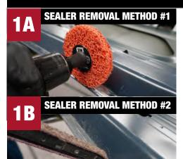
Remove seam sealer using the QLock Strip It Wheel.
