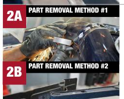
Remove spot welds with spot weld cutter. Remove rivets by drilling or grinding. Remove damaged panel and straighten bent flanges with a hammer and dolly.
